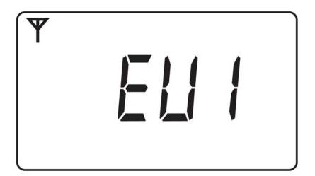
Press [M], and it alternates between EUI (Extended Unique Identifier) and its value
