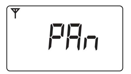
Press [M], and it alternates between Pan and ID (Personal Area Network Identifier) and its value:
