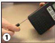
2. Pull battery pack housing away from pump case.
