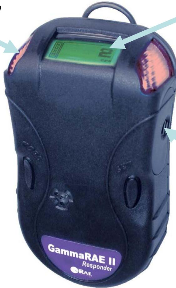
*LCD flips two ways with **SET** button to easily show operation parameters and radiation measurements*
