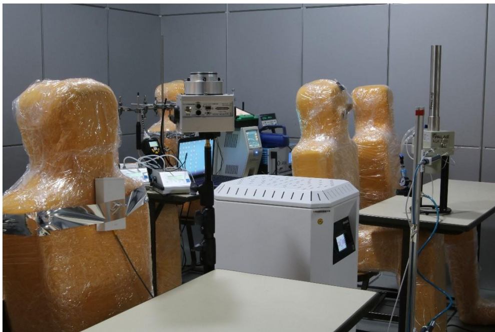
Figure 1: Setup R 150 air purification unit in the IATC with the aerosol generator (dosing unit), sensor technology and air sampler.
